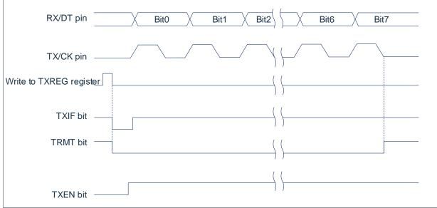
Fig 14-7: synchronous transmit (through TXEN)
