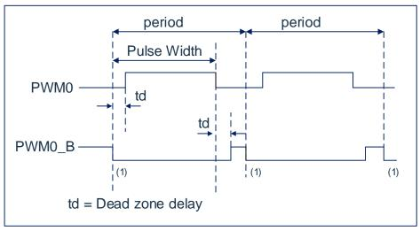
Fig 13-1: Example of PWM dead zone delay output
