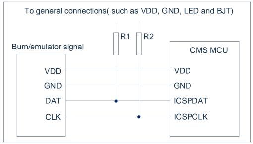
Fig 1-1 : Typical connection for online serial programming
