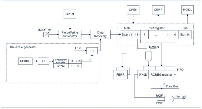
Fig 14-2: USART receive block diagram
