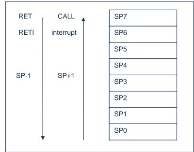
Fig 2-2: stack buffer working principle
