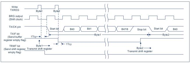
Fig14-4: asynchronous transmit (back to back)
