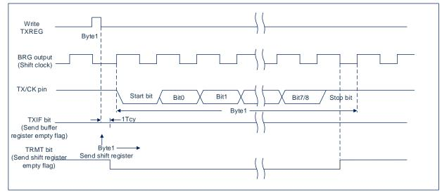
Fig 14-3: asynchronous transmit
