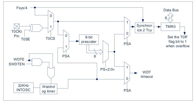
Fig 8-1: TIMER0/WDT mod structure
