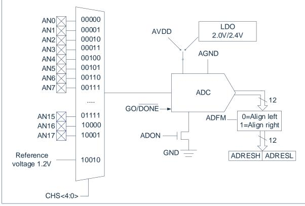
Fig 11-1: ADC structure
