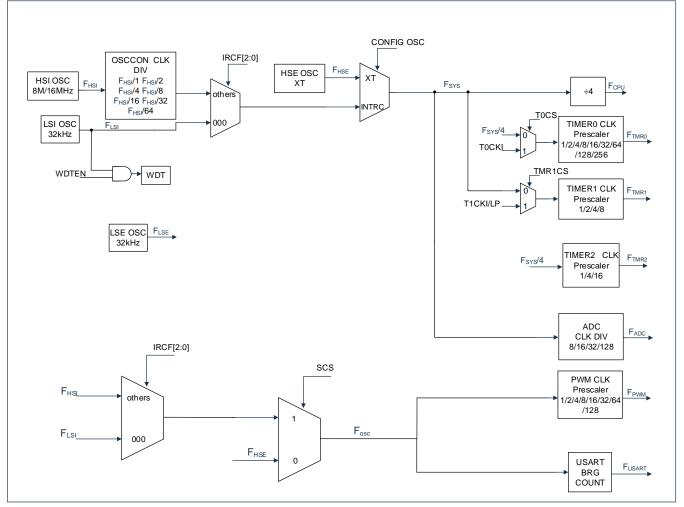
Fig 3-2 : clock block diagram
