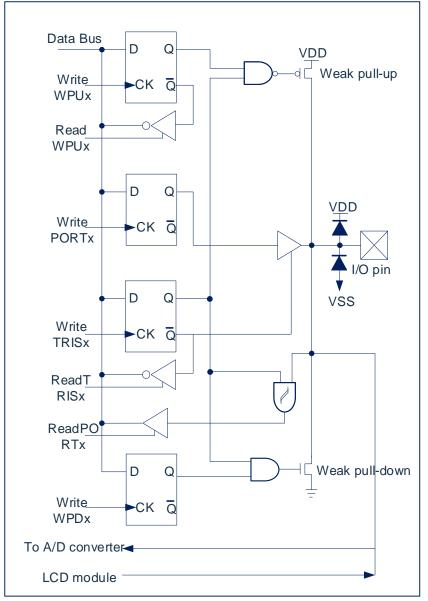
Fig 6-2: I/O port structure—PORTB/C
