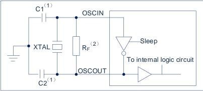
Fig 3-2: Typical XT oscillation
