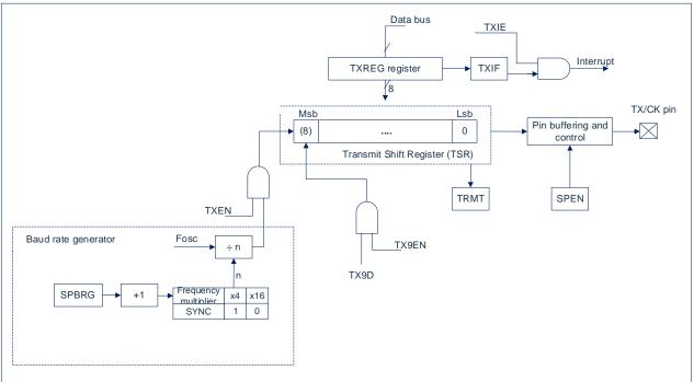
Fig 14-1: USART transmit block diagram
